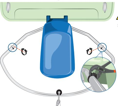
3j. Tighten existing stopper on one side and add one additional stopper next to it.
