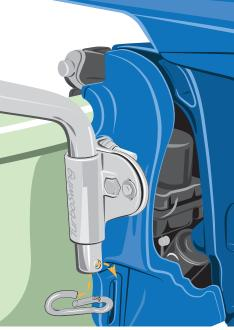
4. Complete your TurboSwing install by inserting the supplied carabiners into the holes at the bottom of the TurboSwing tube. If you are looking for a more permanent installation, feel free to replace the carabiner on either side with the supplied M8x45 bolt and M8 Lock Nut.
