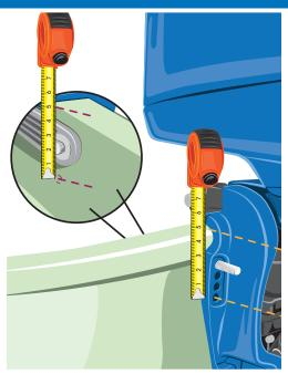
**1d.** Ensure you have space and access inside the transom for your bolt to be inserted using a measuring tape as a guide.
