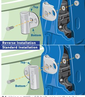
**2d.** Using a M12 x 50 bolt, secure the tube holder to the base plate and tighten using locking nut.
